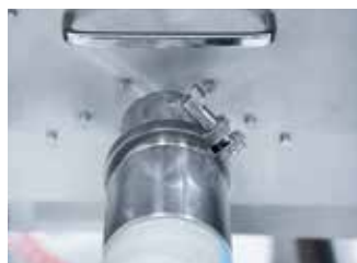
Quick-release pipeline design
